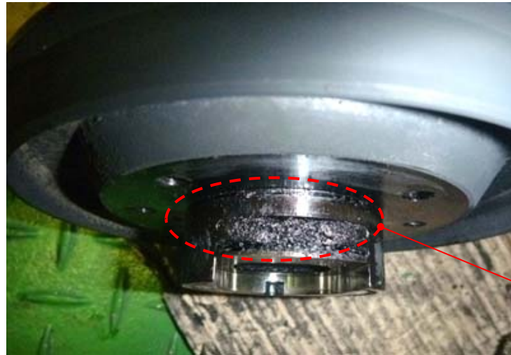
Photo 3. Clogging of Labyrinth Packing LO Return Hole
