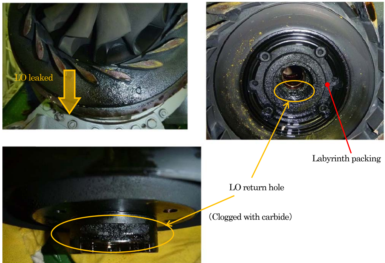
Photo 2. Interior of Turbocharger
